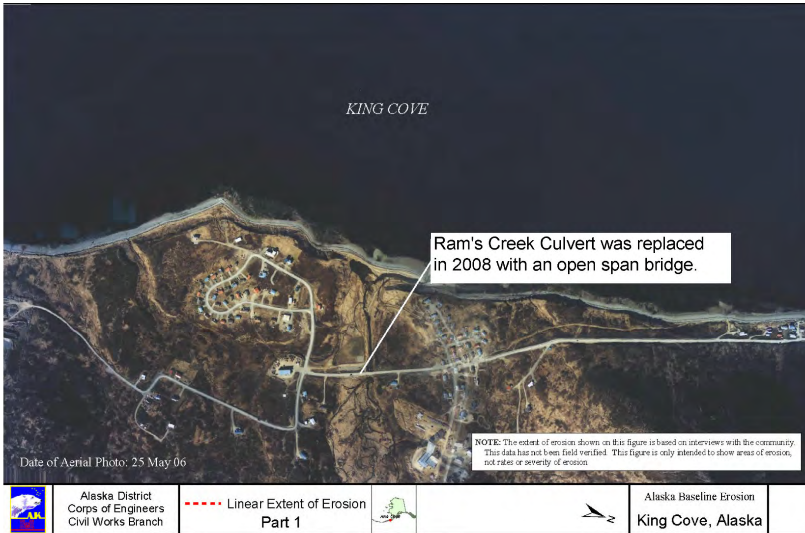
Figure 17. USACE Identified Linear Extent of Erosion in King Cove, Part 1
