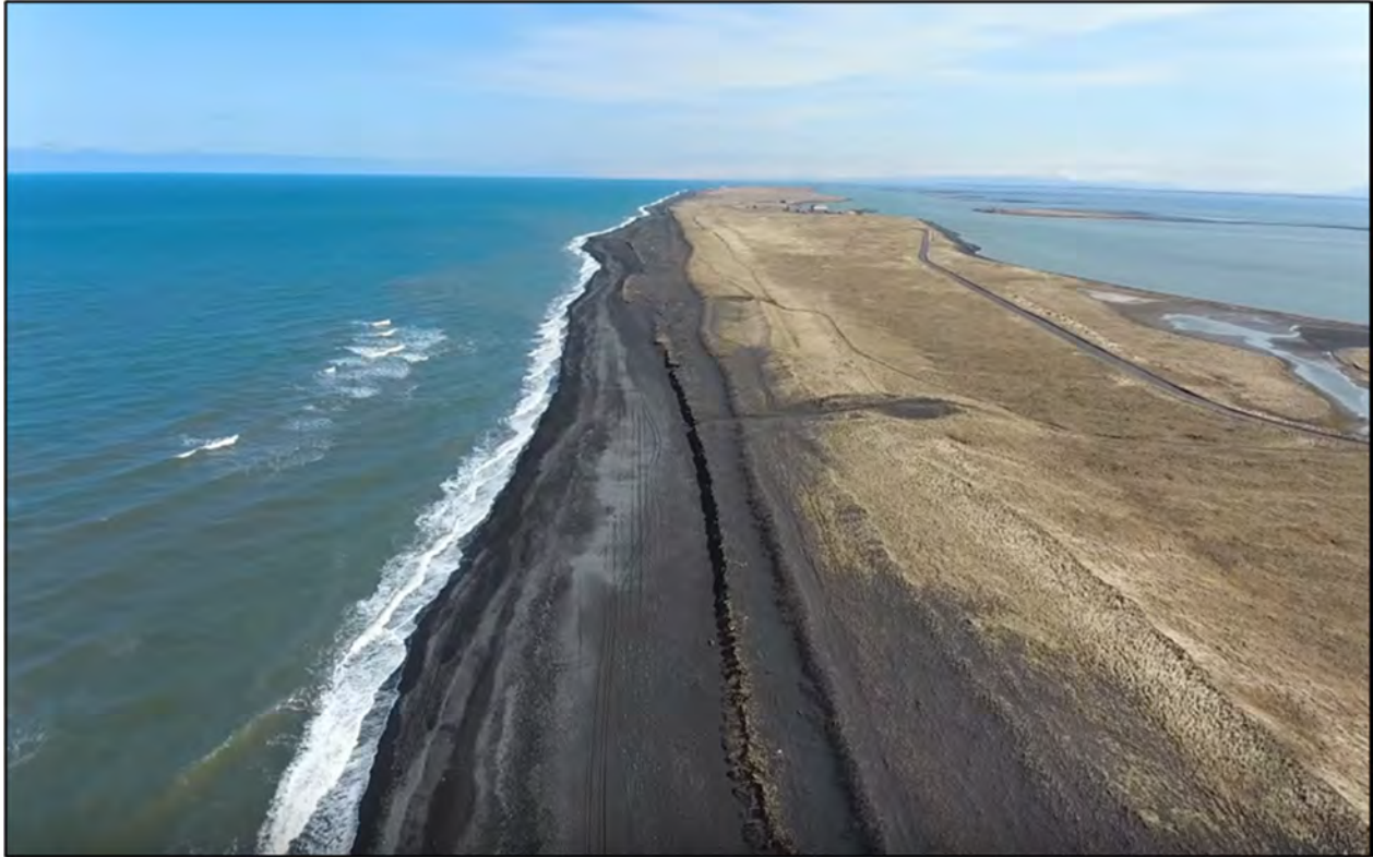
Figure 28. Imagery showing the remnants of overwash deposits along the ocean side of the Nelson Lagoon spit. The road on the right goes from the community to the dock and airstrip. April 2018 by UAF-ACGL.
